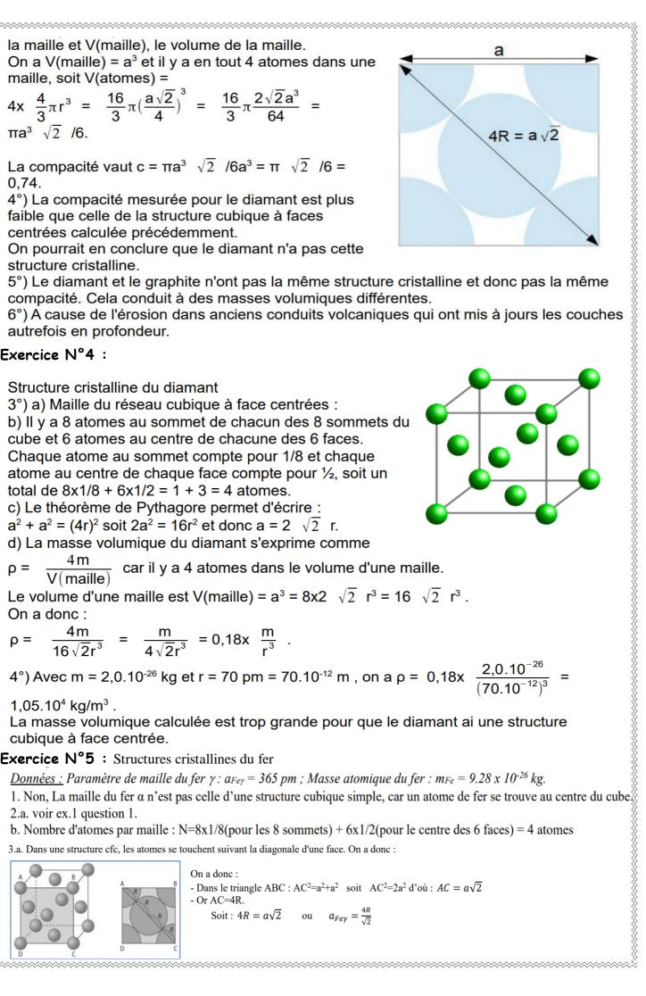
$$C = \frac{4 \times \frac{4}{3} \pi \times R^3}{a^3} = \frac{4 \times \frac{4}{3} \times \pi \times R^3}{\left(\frac{4R}{\sqrt{2}}\right)^3} = \frac{4 \times \frac{4}{3} \times \pi \times R^3}{\frac{64R^3}{2\sqrt{2}}} = \frac{4 \times 4 \times \pi \times R^3 \times 2\sqrt{2}}{3 \times 64R^3} = \frac{4 \times 4 \times \pi \times R^3 \times 2\sqrt{2}}{3 \times 64R^3} = \frac{\pi \times \sqrt{2}}{3 \times \sqrt{2}} = \frac{\pi \times \sqrt{2$$
